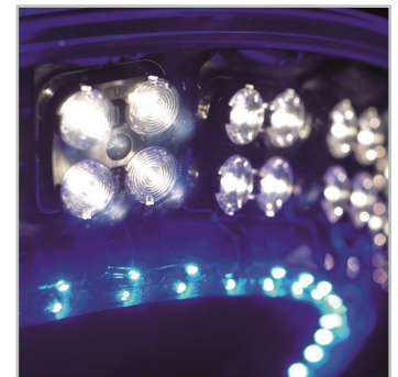
The 64 high-power white LEDs, distributed over 16 modules, are independently oriented and tilted according to the type of light distribution required.
