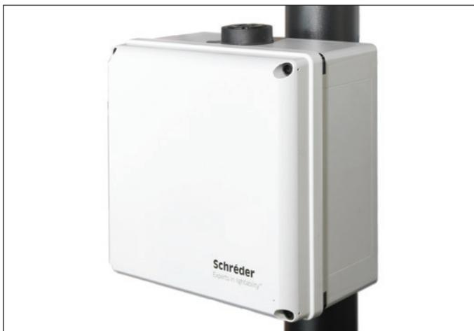
The Schröder ITERRA BASICBOX is the connection hub for the system. All the the drivers' node bus cable connections and the mains power of the nodes themselves are gathered in this cabinet. The Schröder ITERRA BASICBOX is a safe electrical cabinet centralising the wired communication connections (DALI) on the pole. Its purpose is not to feed the drivers' mains input, which should already be done (through the driver boxes).
