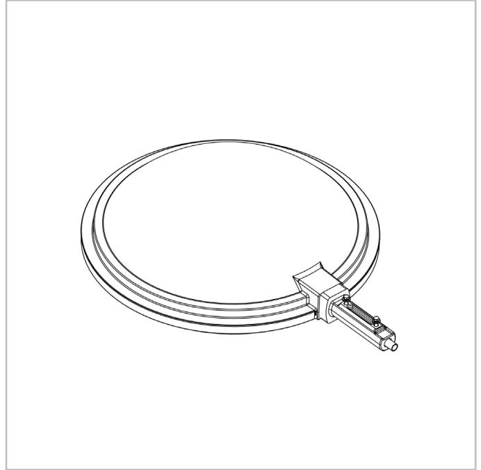
CITEA NG2 | Knuckle joint side-entry enclosing Ø60mm mounting (A6)
